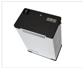
AC Power Switch and Status Screen
